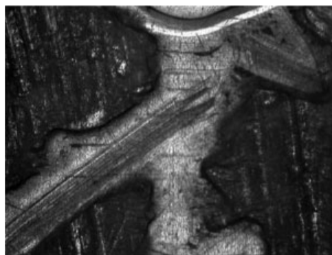
Figure 9 Optical microscopy image (magnification = 5\times , image width = 1.06 mm) of the surface of an HDPE sample photolaminated with AA (dried at 50^{\circ}\text{C} for 2 days after 20 s of irradiation) after a peel test at a crosshead speed of 1 mm/min. The opposing surface looked similar.
